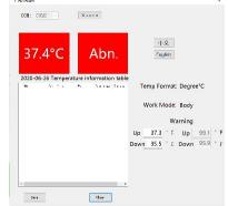
(11)Display specific measurement time of the day and the environment temperature
